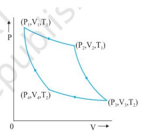
A reversible heat engine operating between two temperatures is called a Carnot engine.
