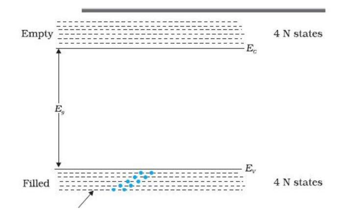
The gap between the top of the valence band and bottom of the conduction band is called the energy band gap (Energy gap  $E_{a}$ ). It may be large, small, or zero, depending upon the material
