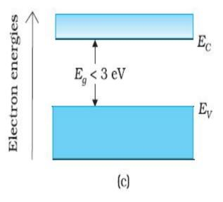
Because of the small band gap, at room temperature some electrons from valence band can acquire enough energy to cross the energy gap and enter the conduction band.
